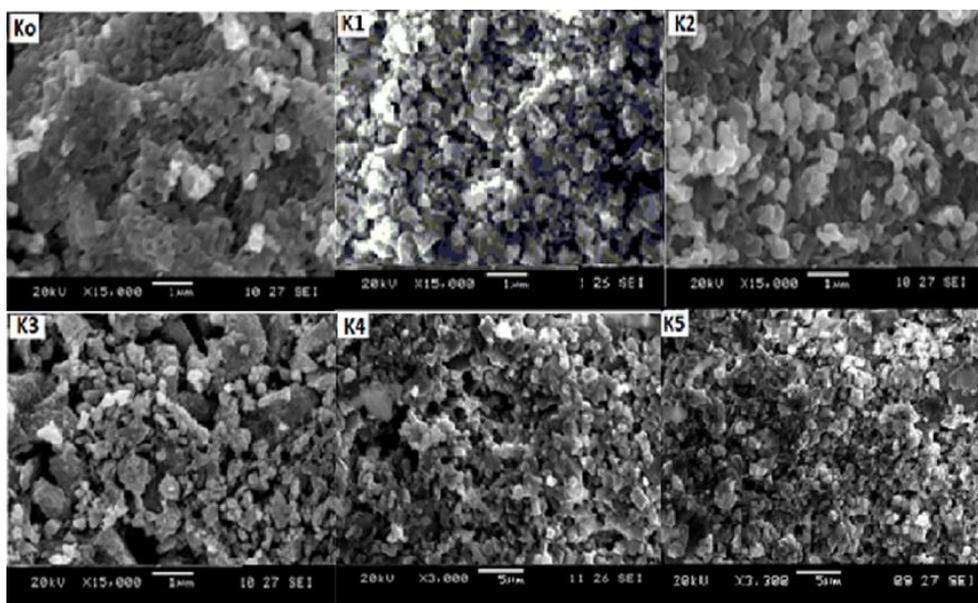
Figure 3.5: SEM micrographs of samples sintered at  $965\pm 5^\circ C$  for three hours
