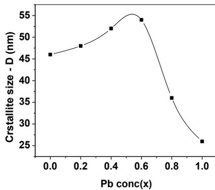
Figure 3.2: Crystallite size ( $D$ ) as function of  $Pb\ conc(x)$
