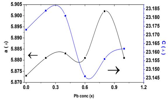
Figure 3.3: Variations in lattice parameters as a function of  $Pb\ conc(x)$
