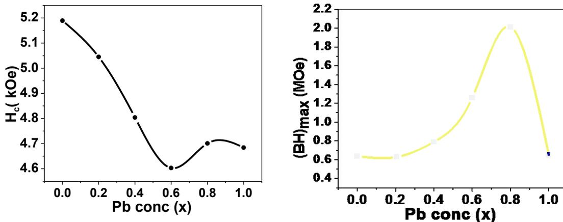
**Figure 4.2:  $H_c$  and  $(BH)_{max}$  as function of Pb conc (x).**
